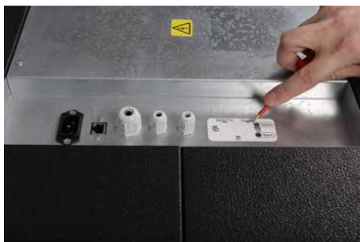
Connections for internet, display, BMS and add-on accessories for the ECO 300/ECO 300 XL.
